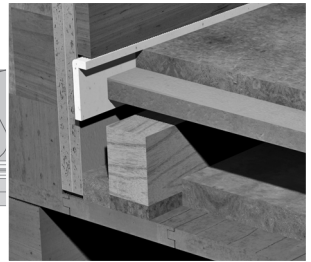
Flanking Strip turned back under skirting and trimmed flush with a sharp knife.
