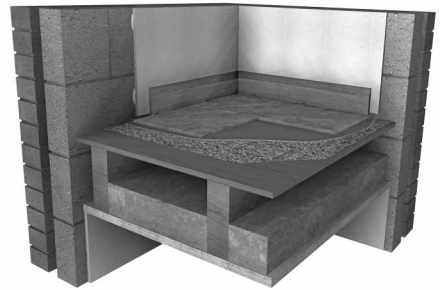
Re-Mat LVT over typical timber subfloor
