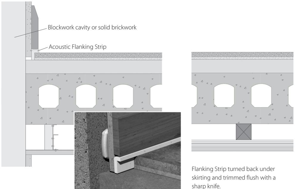
Flanking Strip turned back under skirting and trimmed flush with a sharp knife.
