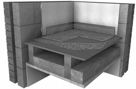
Re-Mat LVT over typical timber subfloor
