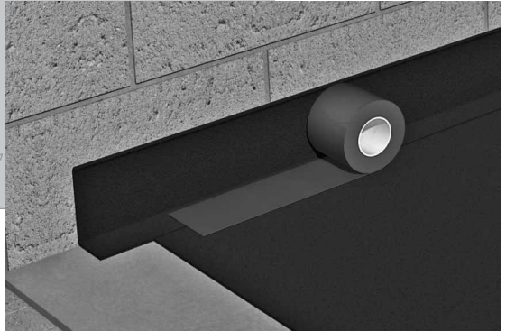
Butt-joint Screedcheck XL9 to flanking strip and seal with 100mm tape.
